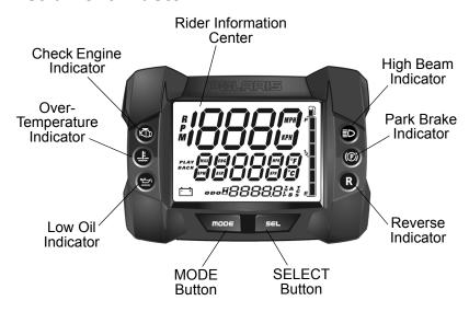
The instrument cluster contains indicator lights and the rider information center. The information center can be controlled by either the MODE and SELECT buttons on the instrument cluster or by the MODE/SET switch on the left handlebar.
